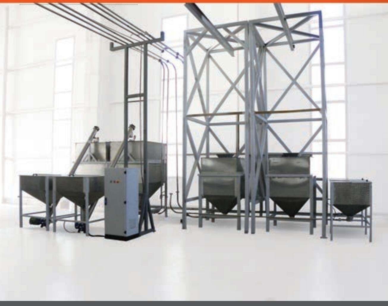
■ This system is suitable for long distance raw material transfer. It can be used for both powder and granule materials. These are customer projects that can be produced in different types.
