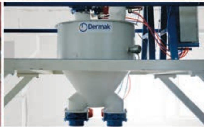
■ Screw feeder loads the material to the mixer and discharges the material from the mixer and loads to silos also feeds extruders.
