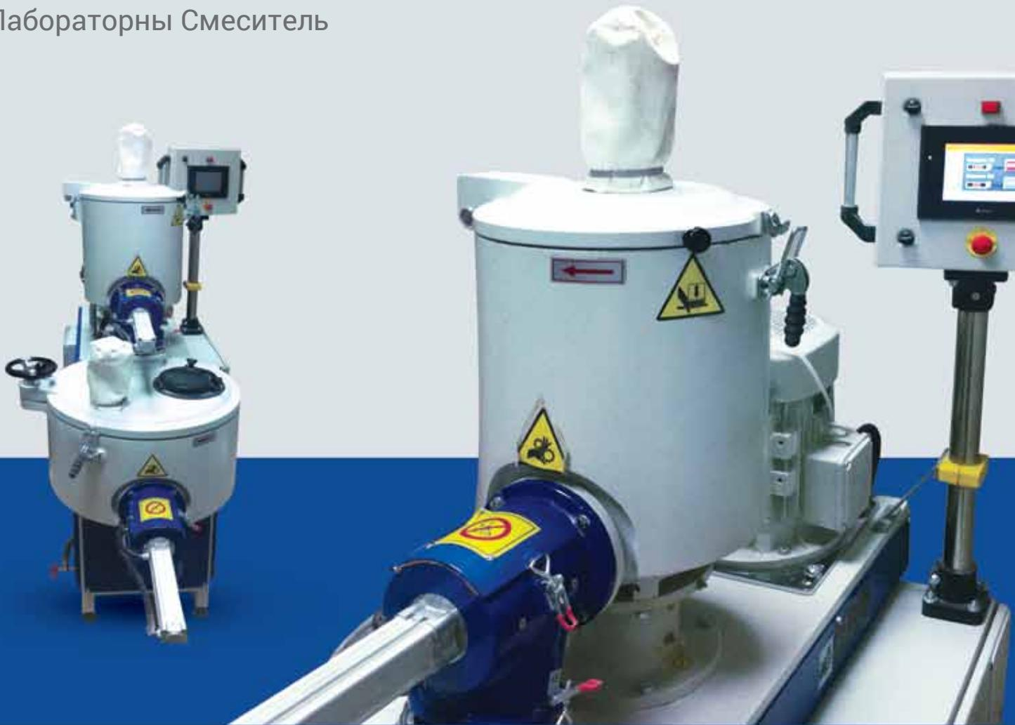
The laboratory mixer (DM-LB) is the smallest in the DER-SAN product line and is therefore particularly well-suited for mixing small amounts. They are often needed for new recipe, production monitoring or for product development, for example. But in spite of its compact size and a usable volume from 10 to 50 liters, the little mixer is extremely powerful and versatile.
