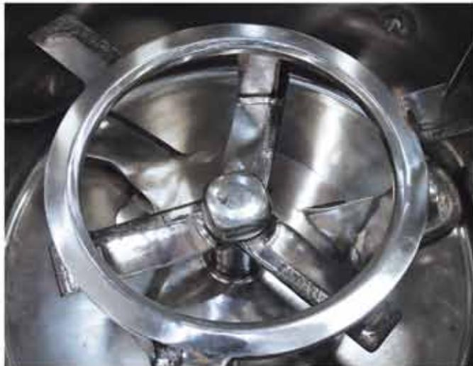
Heater mixer propellers are designed to obtain homogeneous mixing in high circulation. Plated by the tungsten carbide, helps regarding durable of the the propellers. Mainly there is two type of the propellers for mixing of soft and rigid pvc mixtures.
