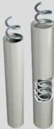
The flexible spiral conveyors, provide an economical means to convey powder or granular material. These conveyors use a stainless steel spiral or steel, enclosed within plastic tubing and they are suitable for transferring material from feed hopper to discharge point. According to the size and capacity Screw conveyors are available in a variety of types.
