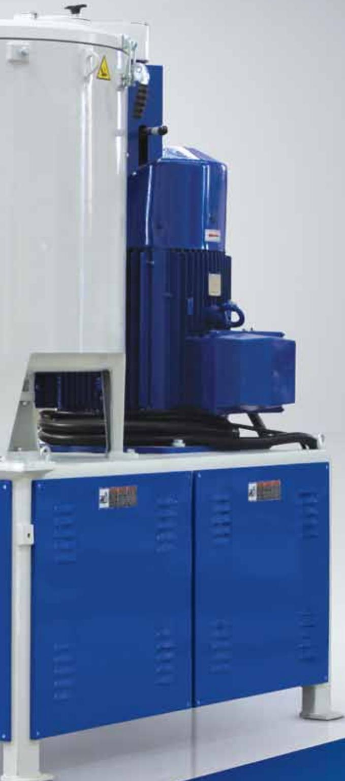
The Heater Mixer (DM-VM) is ideal appliance for the fast preparations of mixes in general and PVC compounds in particular. This types of Mixers are ideal for formulations which are not require cooling process.
