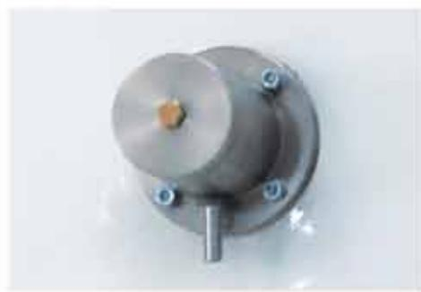
For efficiently transfer of the low weight liquids in to heater mixer we use liquid injection spray. With this device spraying liquid is supplied to the mixer and the raw material is blended homogeneously.
