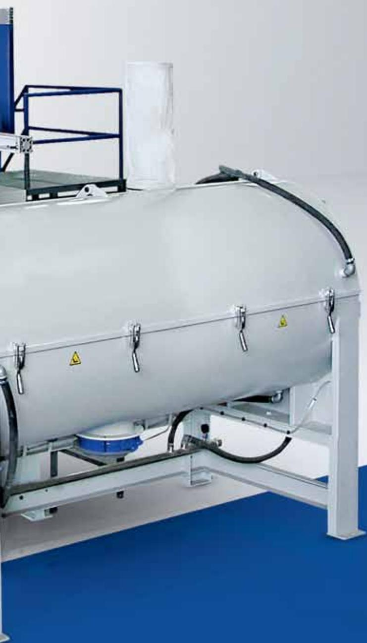
Composite Mixer Wood–Plastic (DM-WPC) ideal for the production of Wood–Plastic Composites typically uses a fine wood waste (cellulose based fiber fillers such as hard-wood, softwood, plywood, peanut hulls, bamboo, straw, etc.) mixed with Plastic. Existing vacuum system to extract the moisture from wood fibers. The moisture content of approx. 16% can be reduced to <1% with vacuum system.
