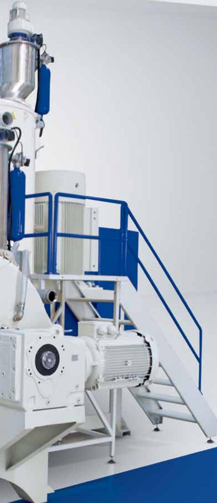
**The Heater – Cooler Combination PVC Mixer (DM-HC)**
